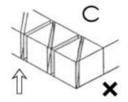
Cutting in direction (C) where the entire light beam runs at 90° to the grain structure should be avoided completely if at all possible.
