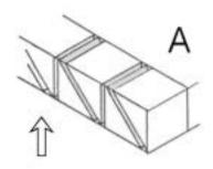
For typical 45° prisms the most obvious use of material is shown in (A) but it should be noted that this is <u>not</u> the optimum orientation.
